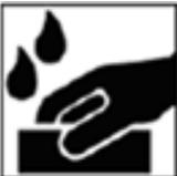
Abrade surface with an ultra fine pad soaked in GenClean silicone remover
