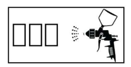
Apply 1 final UNTINTED 2K clearcoat to all panels, simulta-6. neously, as this will have an effect on the final shade and result.
