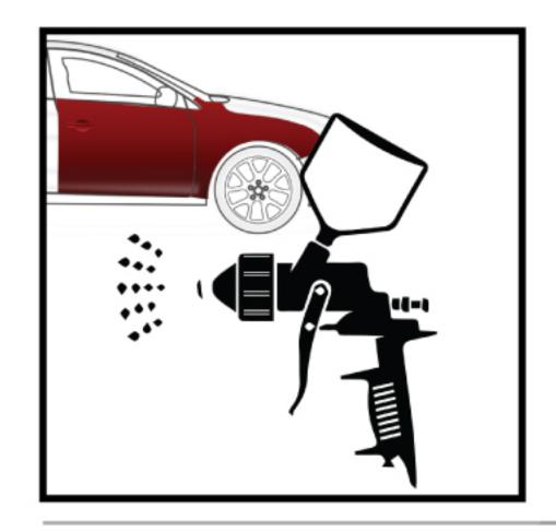
5. Apply 2K tinted clearcoat by overlapping the basecoat area in the desired number of coats as defined by the let-down panel procedure.
