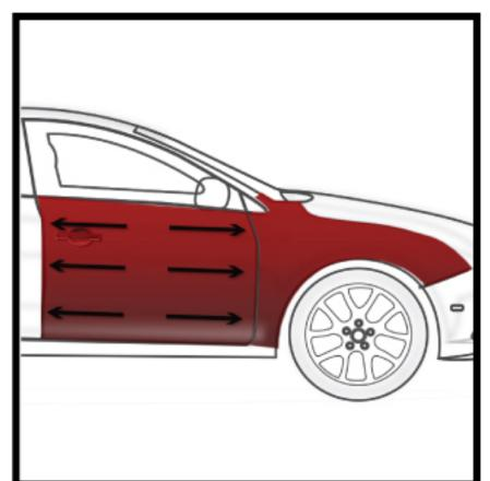
Apply the basecoat to the defined repair area as per technical data sheet.
