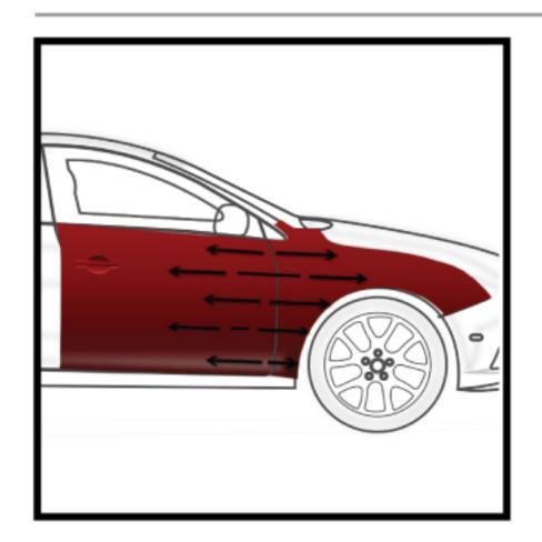
3. Blend the basecoat using the right blending agent from Hymax product list with the right mixing ratio and blending techniques.
